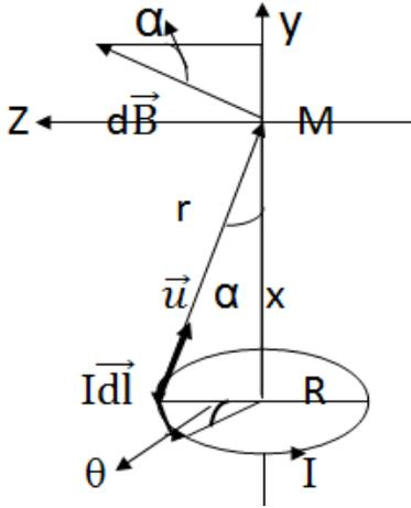
$$dB = \frac{\mu_0}{4\pi} \frac{IdL}{r^2} \quad \text{إذن} \quad dB = \frac{\mu_0}{4\pi} \frac{IdL \sin^2 \frac{\pi}{2}}{r^2} \quad \text{لدينا}$$
