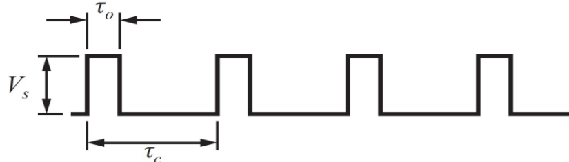
Figure 3 – Description du signal PWM
