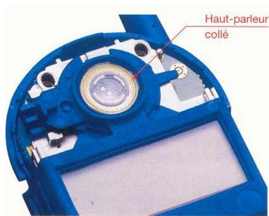
Figure 8: Gluing a mobile phone speaker.
