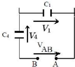
$$V_{AB} = V_4 + V_1 = 2 + 0.8 = 2.8V$$
