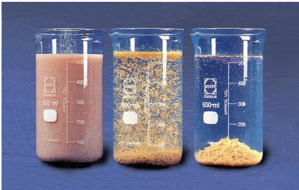
Figure IV.8 : Processus de coagulation-floculation
