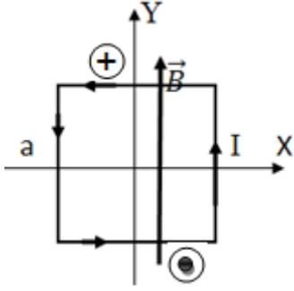
$$\vec{F} = I \int_{+a/2}^{-a/2} dl (-\vec{i}) \wedge \vec{B} \quad \text{ومنه} \quad d\vec{f} = I d\vec{l} \wedge \vec{B} \quad \text{لدينا}$$
