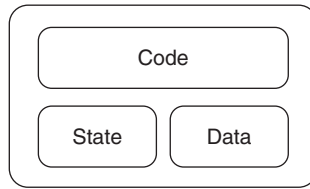
Figure 6.1 Basic structure of a mobile agent
