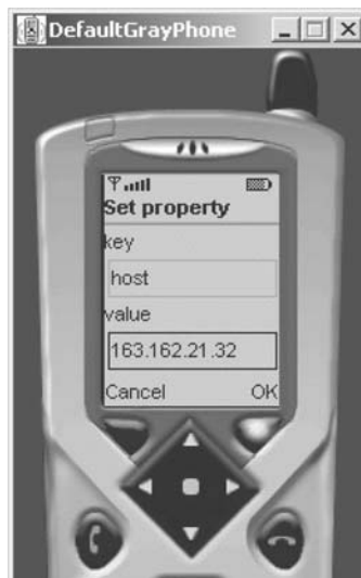
Figure 8.7 Setting configuration options by means of the Config MIDlet
