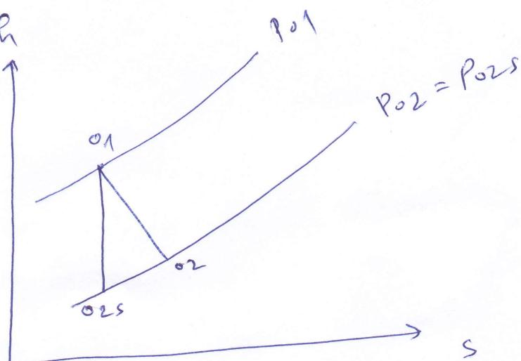
$$N) \frac{T_{01}}{T_{02}} = \left( \frac{P_{01}}{P_{02}} \right)^{\frac{\gamma-1}{\gamma}} \cdot \eta_p \Rightarrow T_{02} = \frac{T_{01}}{\left( \frac{P_{01}}{P_{02}} \right)^{\frac{\gamma-1}{\gamma}} \eta_p}$$
