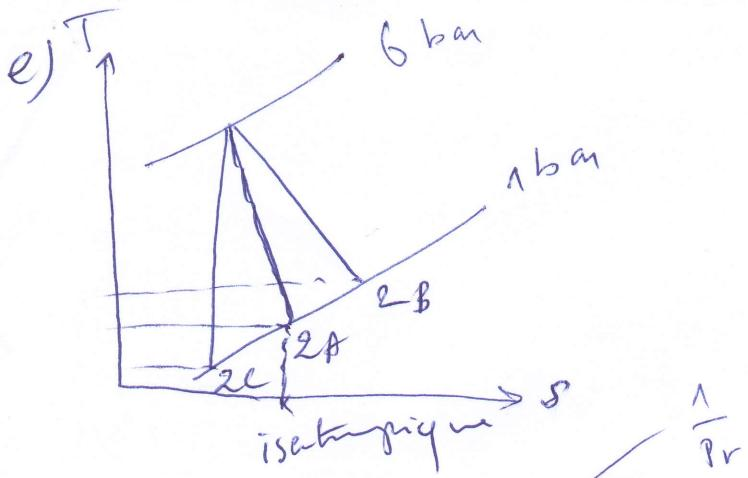
A)  $\frac{T_2}{T_1} = \left( \frac{P_2}{P_1} \right)^{\frac{\gamma-1}{\gamma}} \Rightarrow T_{2A} = 767K$ .
