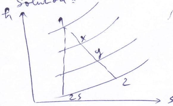
$$\Delta h_T = c_p \Delta T_T = c_p (T_1 - T_2)$$
