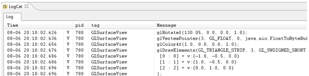
The screenshot shows the LogCat interface with a table of log entries. The table has columns for Time, pid, tag, and Message. The messages are OpenGL ES commands being executed on the GLSurfaceView tag.
